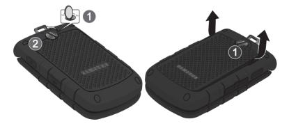
4. Lift the battery up (1) and away (2) from the phone, as shown.
